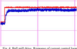
Fig. 4. Ball mill drive. Response of current control loop. Reference step for DC link current:  $I_{DG}(0) = 0.4$ ,  $\Delta i_{DG} = 0.2$ (relative values). Time grid division -0.1 s
