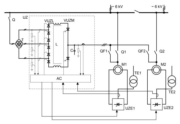
Fig.1. Functional diagram of the drive system: M1, M2 – motors, UZ – CRD, T – transformer, UZE1, UZE2 – exciters, TE1, TE2 – transformers of exciters, Q, Q1, Q2, QF1, QF2 – contactors, VUZL – line converter, VUZM – machine converter, C – filter capacitor, L – DC link reactor, AC – automatic control device
