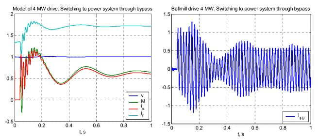
Fig. 6. Processes of drive model and real drive while switching to power system: Model: v – velocity, M – electromagnet torque,  $i_s$  – stator current (module of representing vector),  $i_f$  - excitation current. Real drive:  $i_{sU}$  – instantaneous phase current (relative values)
