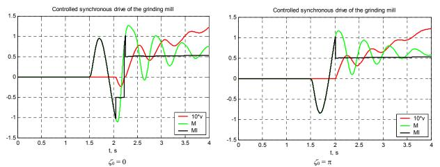
Fig. 3. Processes of drive model for two values of initial angle  $\zeta_0$  between currents vector and *d* axis of motor: *v* – velocity, *M* – motor electromagnet torque,  $M_l$  – load torque (relative values)
